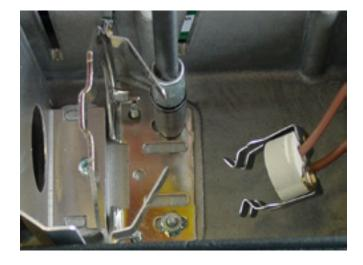
6. Lamp Baffle Removal
