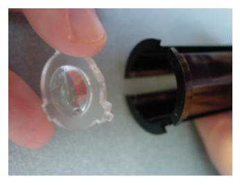
B. Insert the front lens into the main body.
