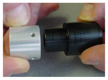
F. Remove the brake from the inside of the insulator.
