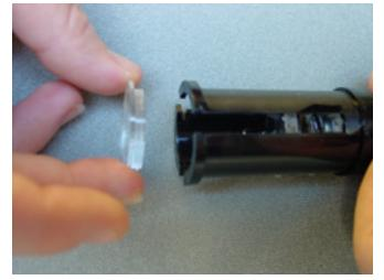
D. Attach the three cam sleeves to the main body. Align the cam slots of the cam sleeve with the front and rear lens tabs.
