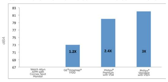
\*In order to collect adequate sound data, a series of floor strips were used to produce continuous, constant and realistic sound. Each stand was assembled per the manufacturers' instructions with the corresponding device attached. Each stand was rolled across the series of floor strips six times at a constant and consistent speed while being recorded. Contact Welch Allyn to obtain full study details.
