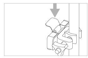
Attach the ventilator to the belt clip on the pole mount by lining up the belt clip with the belt clip sockets on the ventilator. Push the ventilator in towards the vent clip and pole mount until the ventilator audibly clicks into place.
