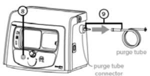
Remove the purge tube connector from the compressor.
