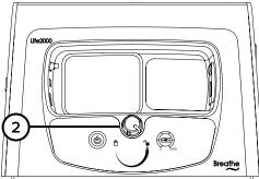
Position the ventilator into the compressor cradle as shown. Push the ventilator into the compressor in the direction indicated by the arrow until it clicks into place.
