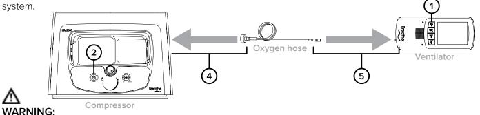
The interface, source gas supply hose, and power cords should be positioned to avoid restricting movement, causing a tripping hazard, or posing a strangulation risk.
