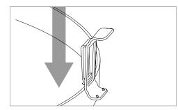
Line up the belt clip with the belt clip sockets on the ventilator. Push in the ventilator towards the belt clip until the ventilator audibly clicks into place.
