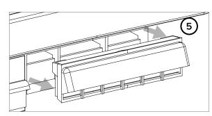
Replace the cooling filter assembly on the back of the compressor by pushing it back into place until it is secure.
