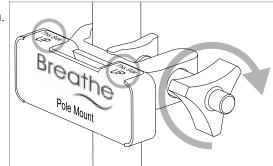
Slide the belt clip for the ventilator into the hole on the top of the pole mount and push down until it is secure.
