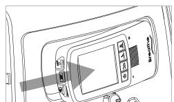
Gently push the top of the ventilator (in the area indicated) until the front of the ventilator is flush with the front of the compressor and clicks into place.
