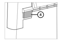
Remove the used filter and inspect the filter.
