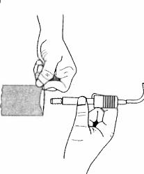
2 Hold open end of sheath and insert light source.
