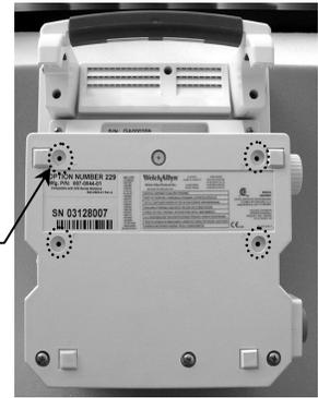
6. Ensure four (4) standoffs on Sub Plate are facing away from the monitor (see below), and fasten Sub Plate to rear of monitor with four (4) #6-32 x 3" PHMS as shown below.
