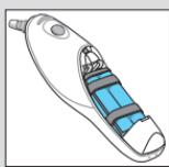
The Base Station is supplied with 1 rechargeable battery pack. To make use of the charging function place the rechargeable battery pack in the battery compartment of the thermometer.
