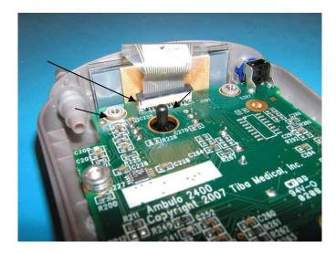
7. Remove the 2 screws that connect the PCB to the top cover. You can now remove the PCB from the device.
