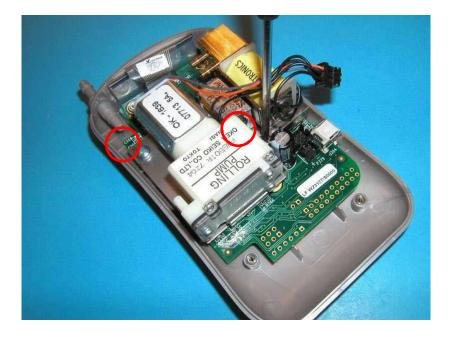
5. Gently lift the right side of the electromechanical assembly (the side opposite the air socket) until you feel the manifold disconnect from the pressure sensor port on the PCB. The assembly will now be secured only by its connection to the air socket.
