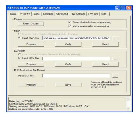
6. After programming is completed, note the firmware version provided at the bottom of the programming software window.
