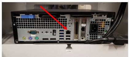
Connect the LAN isolator adapter to the Network Port (RJ45 connection) shown above right and connect the institution LAN cable to the isolator. Then use the Velcro provided to attach the isolation adapter in a convenient location, as shown above left.
