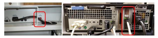
If using a Z200+ with an integrated network (LAN) connector, connect the ethernet crossover cable from Z200+ thermal printer to secondary LAN card on the PC following the channels and cutouts. The LAN port used for the Z200+ should be labeled "Z200+" from the factory. (LAN connections shown above)
