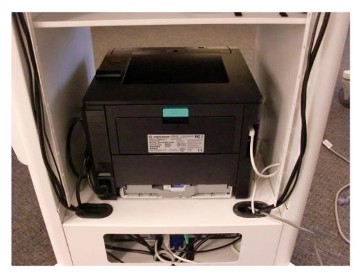
The cart back panel has been removed for easy access to the printer back during installation. This is done via removal of two M4  $\times$  6 mm screws at the top of the panel.
