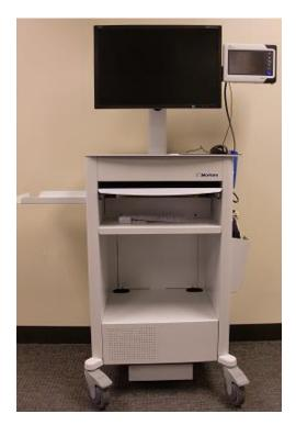
Finished Cart with the Z200+ Thermal Writer configuration, 24" LCD, SunTech Tango M2 BP monitor and Computer components installed.
