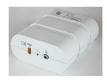
Trigger module front for AM12 connection to the ECG A connector and one analog out connection.
