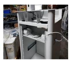
The modules are installed and secured with (2) screws in the upper corners of the storage compartment.
