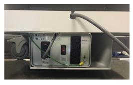
Connect the main AC Power Cord to the Isolation Transformer AC inlet as shown.
