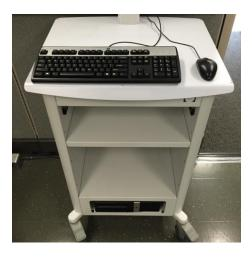
Place keyboard and mouse on work surface. Route cables through monitor mount, and attach the connector to the computer back.
