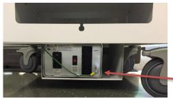
Insert the Isolation Transformer with the power entry module facing the back. Carefully slide the Isolation Transformer into the bottom opening on the back of the cart being careful not to scratch the cart.
