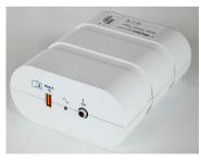
XScribe AM12 patient cable must be connected to ECG A USB connector on the Trigger Module front. One active analog output connector (→ 1) is also on the front.
