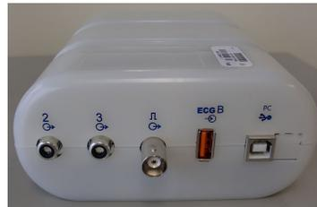
The module back provides two analog output connectors (⊕ 2 and ⊕ 3 are currently non-functional) and one TTL (⊕ TTL) output connection.
