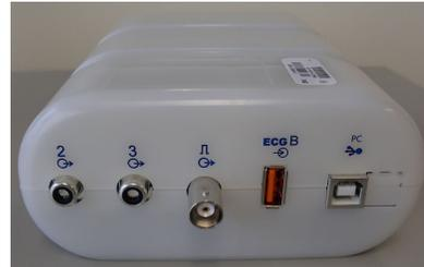
The module back includes two non-functional analog output connectors (2 and 3) and one TTL output (square wave symbol) connector.
