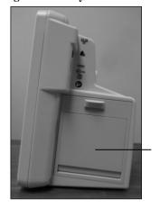
The right side of the Surveyor S12 may contain the optional integrated dual channel thermal recorder (1).
