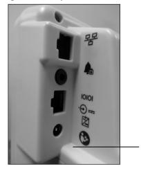
The top corner of the back of the Surveyor S12 and S19 contains the communication ports, an opening for the audio speaker as well as a connection for CO<sub>2</sub> exhaust.
