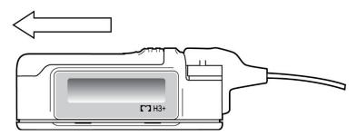
To close the battery door, place the battery door on the H3+ as shown below and slide the door in the opposite direction until the door snaps into place.
