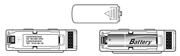
*NOTE:* The H3+ requires a fully-charged battery to record a 24-hou or 48-hour session. Always use a new battery to ensure operation.
