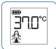
If the thermometer is unstable or patient is moving during the measuring process, the device will beep, the green ExacTemp light will flash and POS (Position Error) will flash on the display. **Be sure the device is stable and restrict patient movement for the next measurement. Change the probe cover to reset.**
