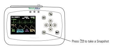
Press 🛅 to capture a 21-second period of numeric and waveform patient data. The monitor captures the 14 seconds preceding and the 7 seconds following the button press.
