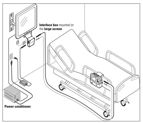
Figure 15. Interface box mounted on the large screen
