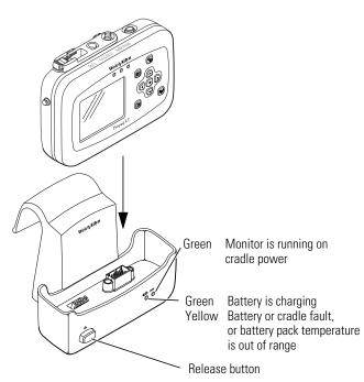
A steady yellow light indicates a problem with the battery or the cradle (contact a qualified service technician) or that the temperature of the battery pack is out of range.
