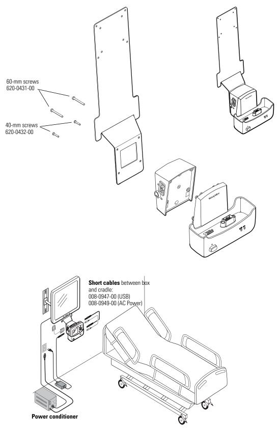
Figure 26. Mounting the interface box and the cradle on the large display mounting bracket
