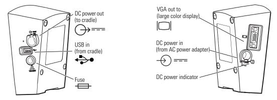
When the interface box is attached to the cradle, the default power and USB cables connect the interface box and the cradle. (See Figure 17 on page 23.)
