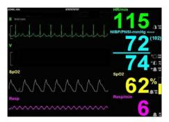
Leads I, II, and III are viewable. The waveform for the lead selected at the monitor is displayed on the large color display. Lead V cannot be displayed.
