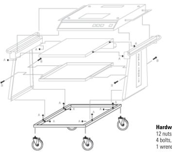
Hardware included: 12 nuts, 1/4-20 flange whiz (60627) 4 bolts, 1/4-20 x 1/2" (130241) 1 wrench, stamped flat metal (48807)
