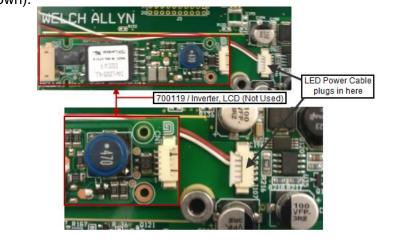
When replacing the LCD in a device that was manufactured after June 2014, there will be no inverter board installed. The LED Power Cable will plug directly into connector J107 (as shown).
