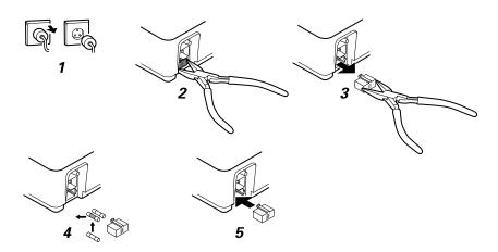
If either fuse is dark or has a broken wire, replace the fuse. Line up the fuse case with the opening; it goes in only one way.
