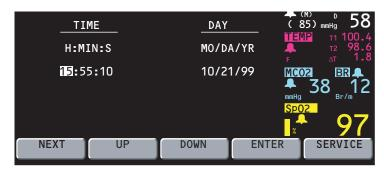
2. Press **NEXT**, **UP**, and **DOWN** as needed to set the time and date. Then press **ENTER** to store the new time and date.
