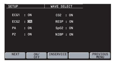
You can turn on all waveforms, but only the first four waveforms selected as ON in the Wave Select window are displayed. You cannot turn off the ECG1 waveform.
