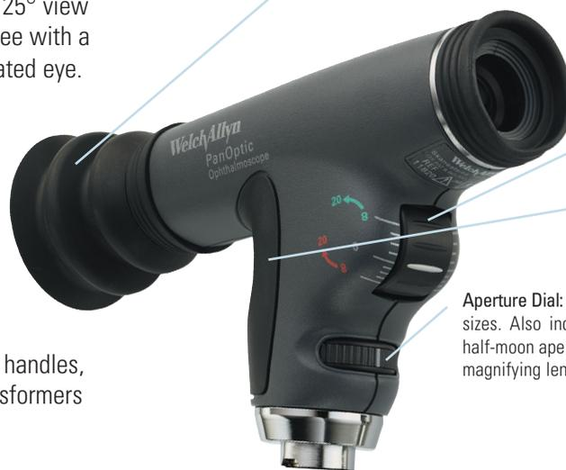
**Patient Eyecup:** Establishes and maintains proper viewing distance, provides image stability, serves as a pivoting point for panning around the retina, helps with orientation and screens out ambient light. The eyecup is cleanable and reusable.
